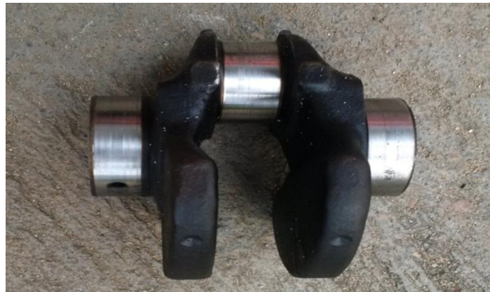
Figure 1. Specimen A showing the failed crank pin journal
