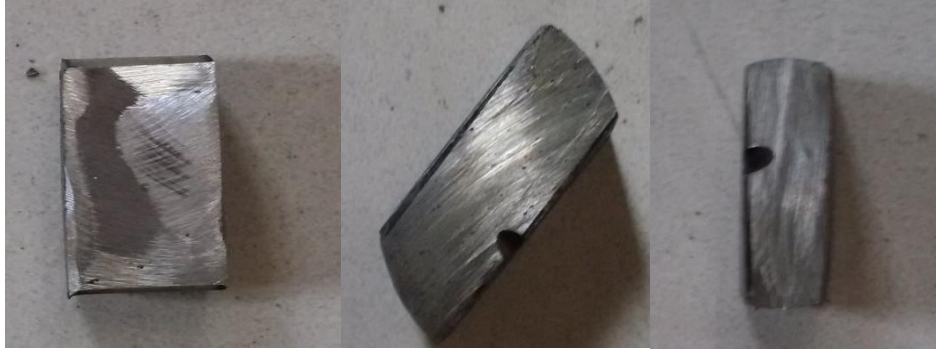
Figure 4. Samples machined out from the crank-pins
