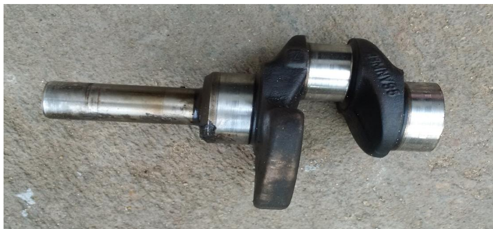
Figure 3. Specimen C showing the failed crank pin journal
